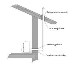
If the gas exhaust pipe is installed as in the drawing on the right, a rain protection cover will be needed in addition to the requirements listed above.
